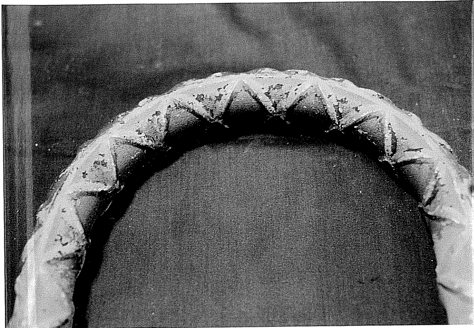
Figure 4.3: Coating Flaked During Bending
